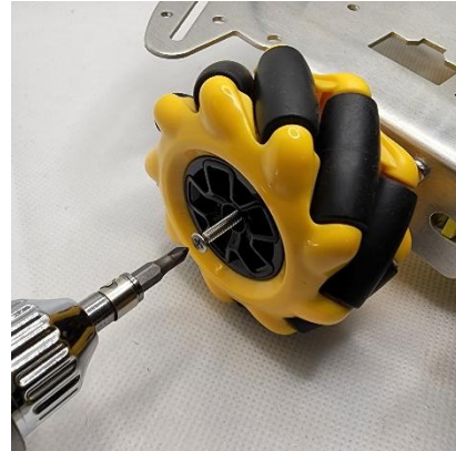
Image 2: Connecting the wheel and motor
